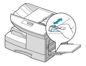
Make sure that you have not loaded too much print media. The stack should be under the max. fill line. The print media buckles if you load a stack that is too deep, or push it in too far.
